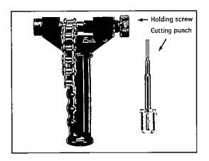
① Insert the chain on the chain cutter and tighten the holding screw.
