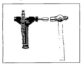
(3) Hammer cutting punch several times, then be sure to tighten the holding screw again. Then hammer repeatedly as photo till the pin pops out.
