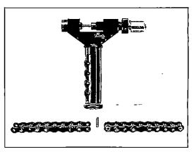
4 After the pin pops out, release screw and remove the chain.
