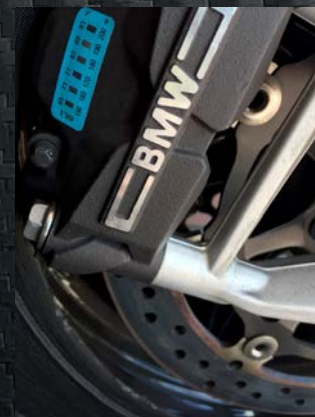
Brake caliper prepared with temperature stickers.
