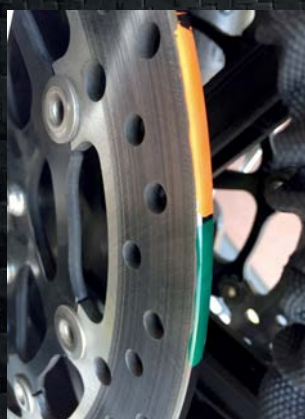
Brake disc prepared with Thermal Paint GREEN (430°C) and ORANGE (560°C).
