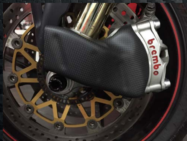
Brake caliper air duct.
