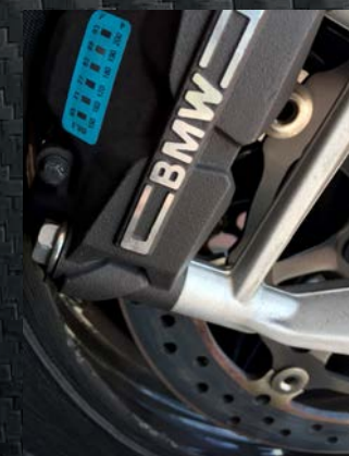
Brake caliper prepared with temperature stickers.
